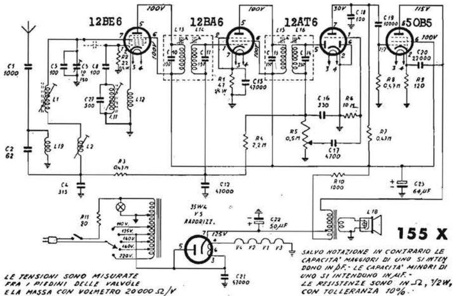
LE TENSIONI SONO MISURATE FRA I PIEDINI DELLE VALVOLE E LA MASSA CON VOLMETRO 20000 Ω/V
